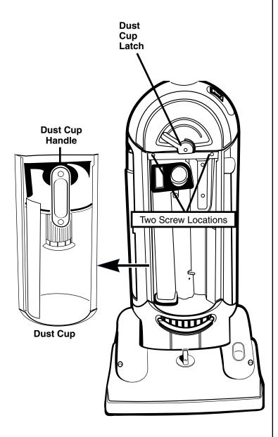
Remove dust cup from unit to expose the two screw installation locations. Release the dust cup by rotating the dust cup latch to the left. Pull out and up on the dust cup handle to remove from unit.
